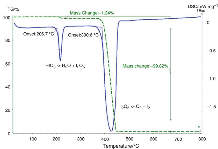
**Fig. 2** Heat flow and mass loss curves for  $Al_2O_3$  and  $I_2O_5$ , experiments performed in an Ar environment at a heating rate of  $10\text{ }^{\circ}\text{C min}^{-1}$
