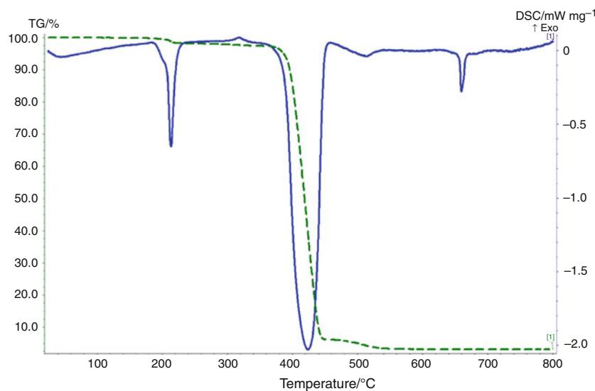
**Fig. 4** Nanometer scale Al powder and I<sub>2</sub>O<sub>5</sub> with an equivalence ratio of 0.4, experiments performed in an Ar environment at a heating rate of 10 °C min<sup>-1</sup>
